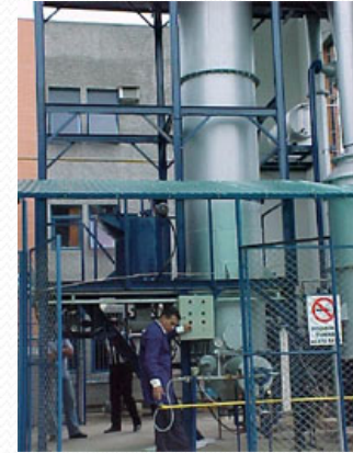
Figure 2– View of gasifier biomass feeder silo and the gasifier bed section.
